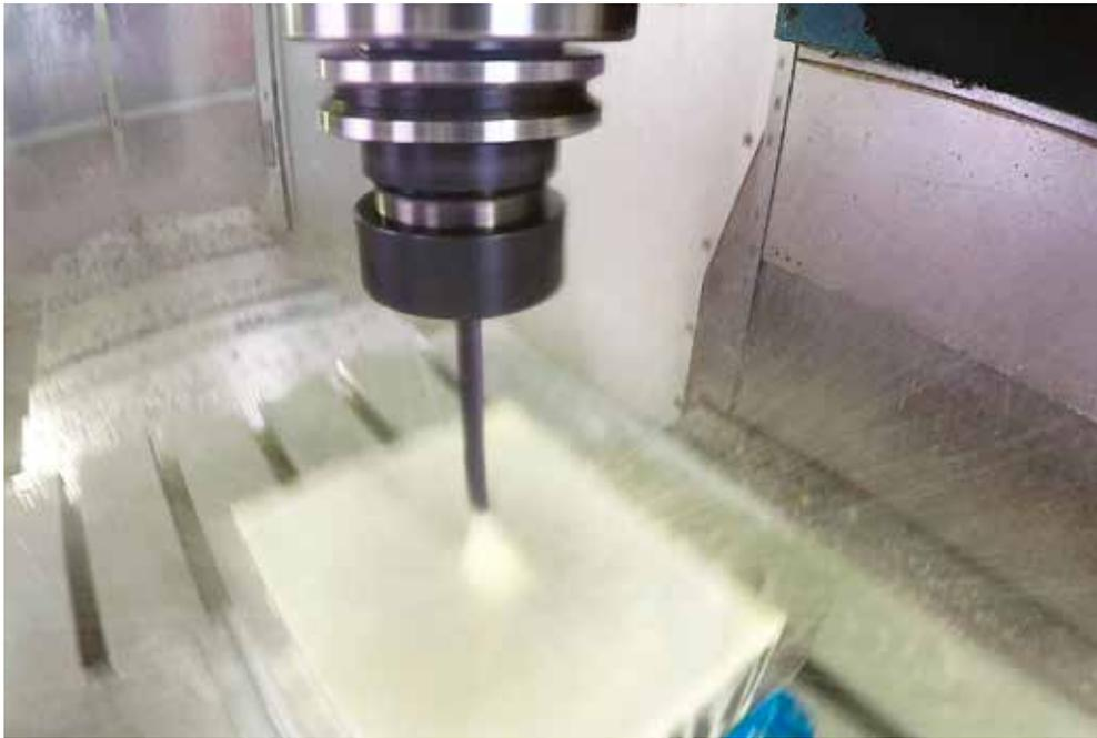
The ROMI D1000AP channels coolant through a high-speed carbide drill bit to flush out chips.
